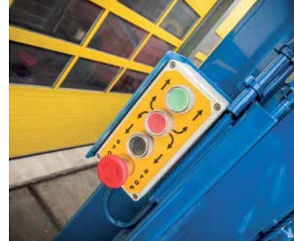
Moving switch box on left slider, including emergency stop.
