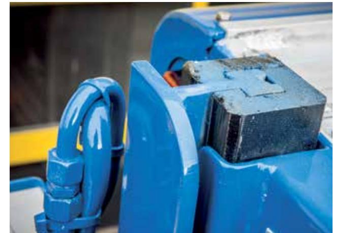
The unique Berdex powered tailgate design with its slide pads features as few moving parts as possible. This ensures dependable usability.
