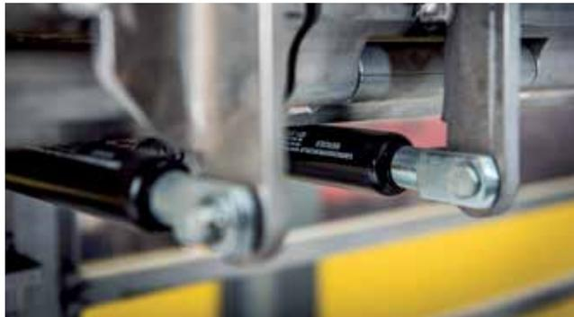
Light controls for folding floor components due to gas-spring support.
