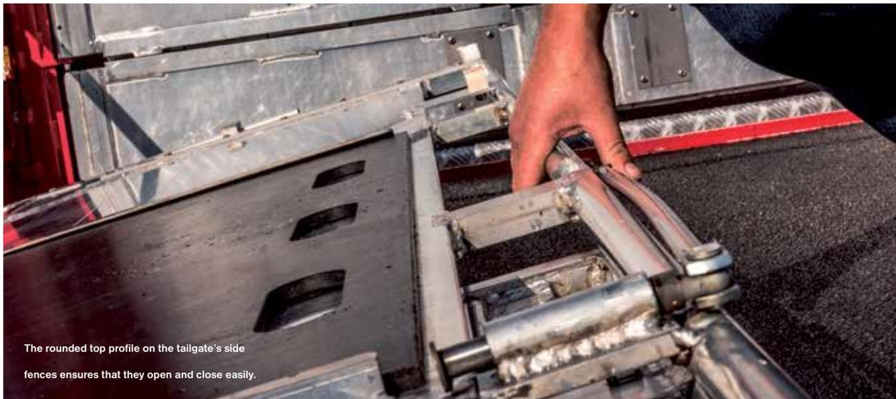
The rounded top profile on the tailgate's side fences ensures that they open and close easily.
