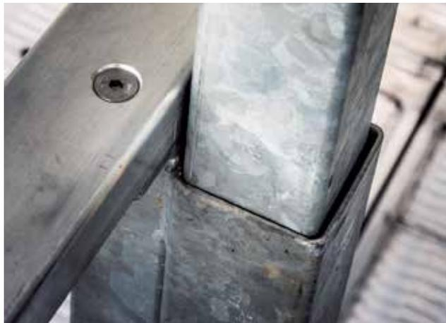
Detailed view of umbrella hitch support. Riser with hidden hydraulic cylinder. Unique Berdex design with barely any moving parts.
