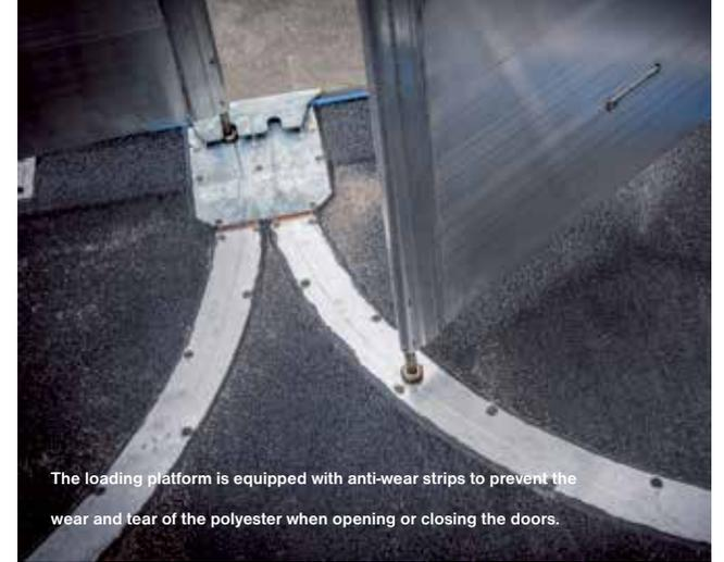
The loading platform is equipped with anti-wear strips to prevent the wear and tear of the polyester when opening or closing the doors.
